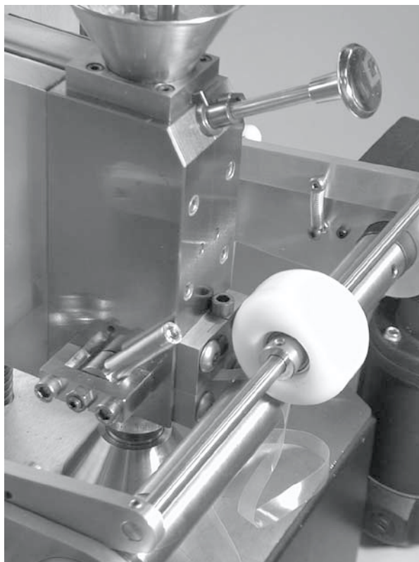
Film being extruded using the film attachment. The optional continuous extrusion attachment is also shown in this picture.
