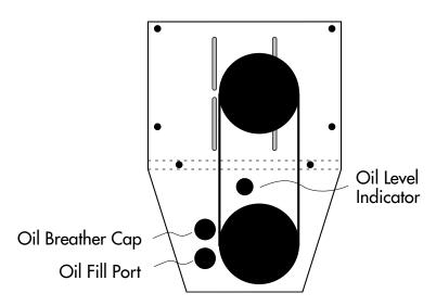
Additional oil might be obtained through DACA Instruments. To replace the oil the chassis must be removed to access the drain plug in front of the gear box. For instructions contact DACA Instruments.
