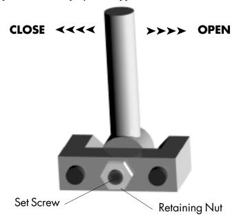
WARNING: DO NOT PUSH THE VALVE FROM INSIDE. Doing so will damage the inner surface of the valve and allow the sample to leak through the exit port during tests.
