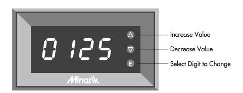
As received, the MicroCompounder has its speed set to 0000. As soon as AC power is turned on, the speed controller will be operating. When the speed controller is in its operating mode, press the ENTER push-button (**E**) once to get into the speed setting mode. Only in this mode do the digits in the display flash on and off. Flashing indicates which of the digits is able to be changed to a new value or have its value 'ENTER'ed before proceeding to the next digit.
